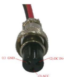
Power & ACC cable
