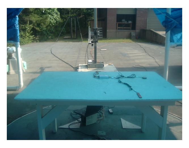
Figure 5 Radiated Emissions (Rear View)
